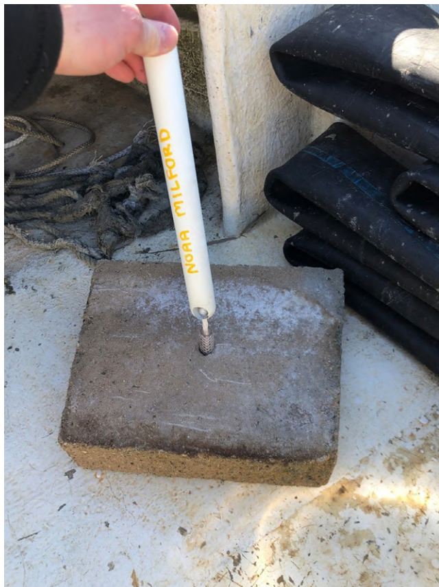
Figure 3. Tiltmeter setup for deployment at each farm site.
