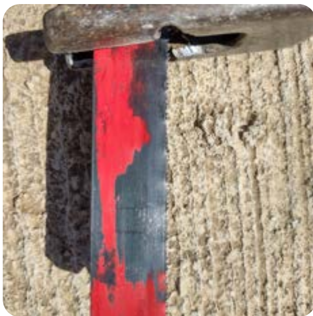
A new blade will make all the difference no matter which saw you use. Small teeth work best for cutting metal.
