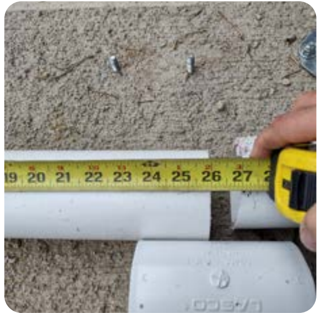
Cutting PVC pipe air line. A circular saw, reciprocating saw or hack saw will work well. Wear eye protection!
