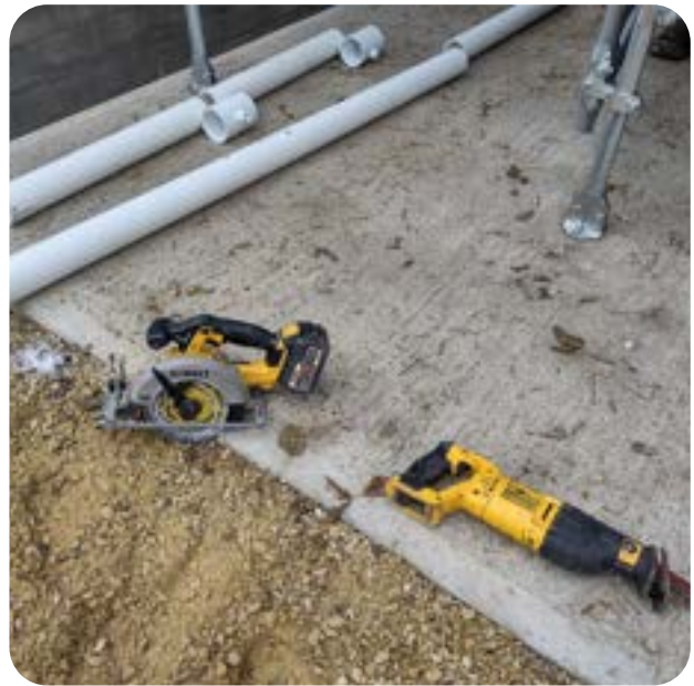
Cutting PVC pipe air line. A circular saw, reciprocating saw or hack saw will work well. Wear eye protection!
