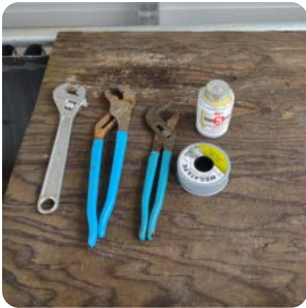
Tools needed to install stall-cocks- wrench or channel locks, Teflon tape and/or thread sealant
