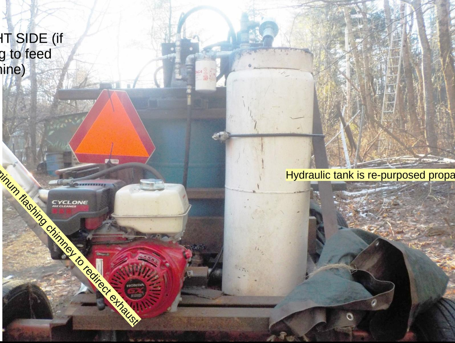
Hydraulic tank is re-purposed propane tank
