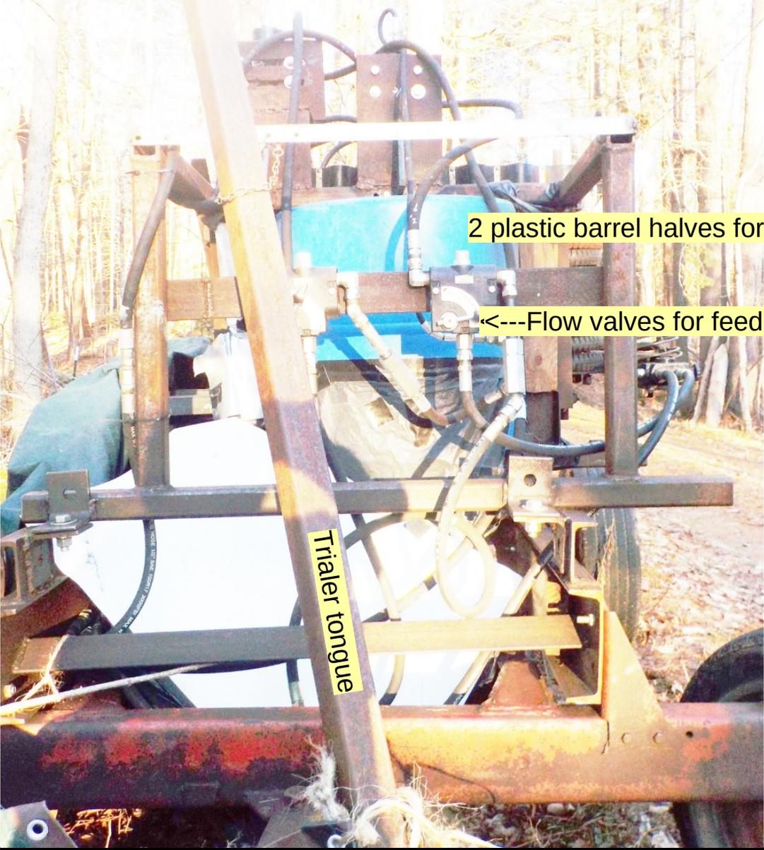
2 plastic barrel halves for flail housing
