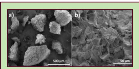
SEM Micrograph of SCG at 200 (a) and 2,000 (b) magnification (Ballesteros et al., 2014)
