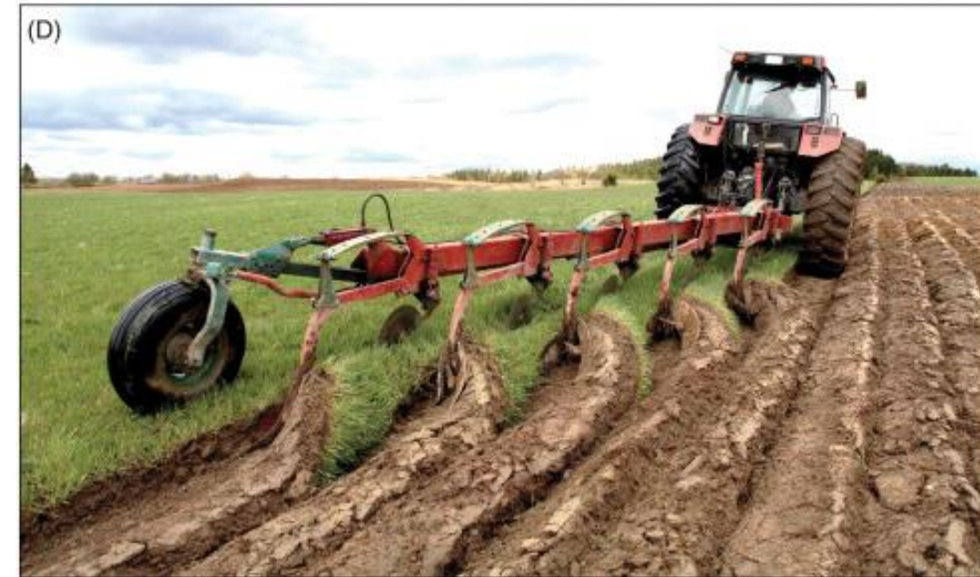
Pictured: A moldboard plow. Alan Joseph Franzluebbbers, in Principles and Applications of Soil Microbiology (Third Edition), 2021.
