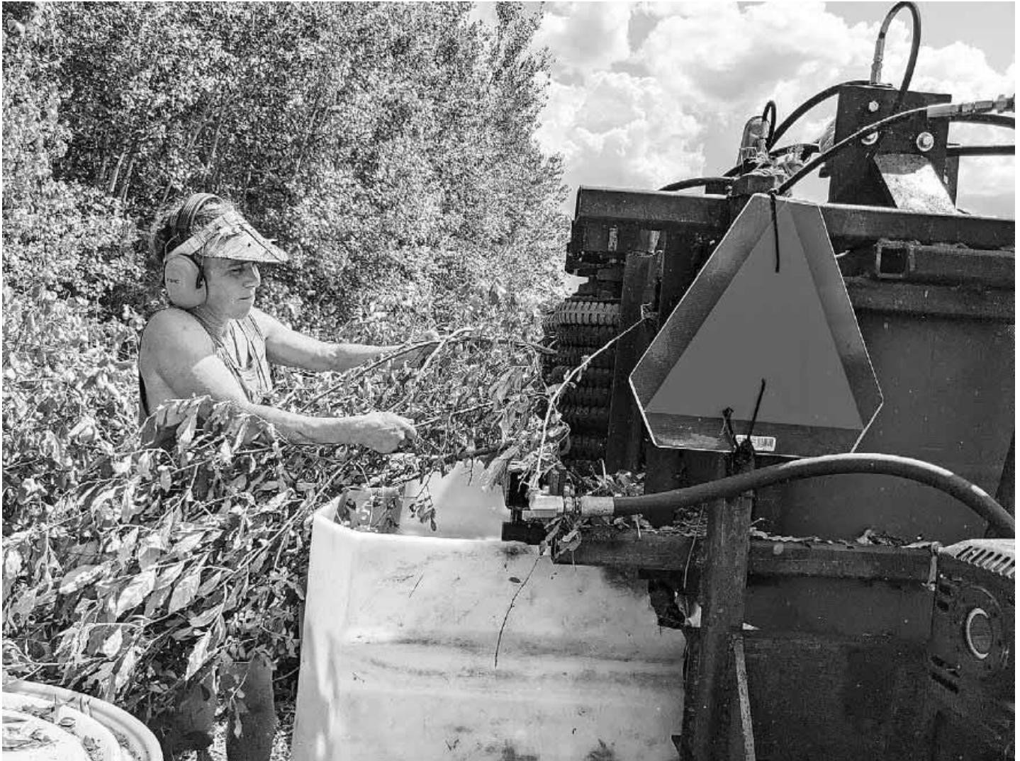
Shana Hanson feeds autumn olive boughs into a prototype leaf-separating machine. PHOTOS BY ETHAN ANDREWS
