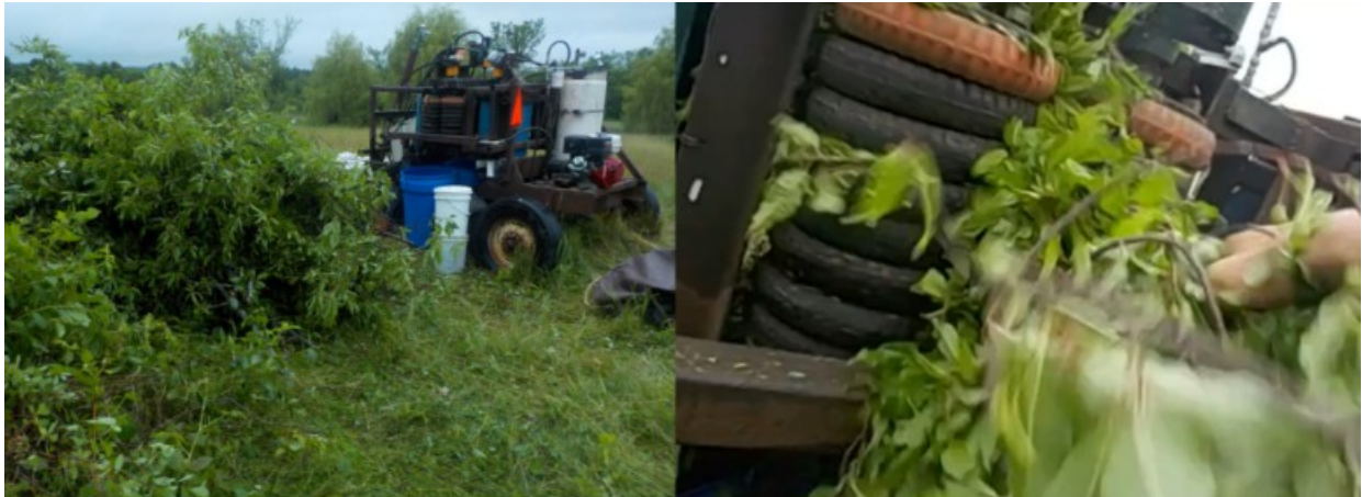
Figure 1. Chain-flail leaf-separator prototype in operation.
