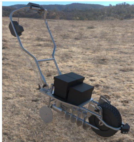
Fig. 12 The Auger Electric Tiller, with improvement. It features real-time feedback on vibration, sound, and operational metrics, along with visual and auditory warnings followed by a safe shutdown mechanism to enhance usability and safety for farmers.
