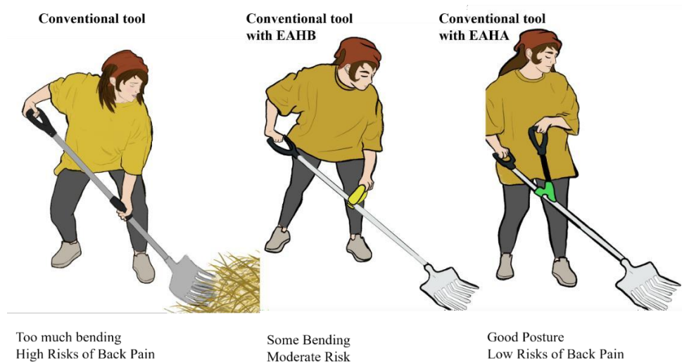
Fig. 6 Comparison of postures: User 1 (left) with a conventional tool shows high back pain risk; User 2 (center) with an EAHB handle shows moderate risk; User 3 (right) with an EAHA handle shows good posture and low back pain risk.
