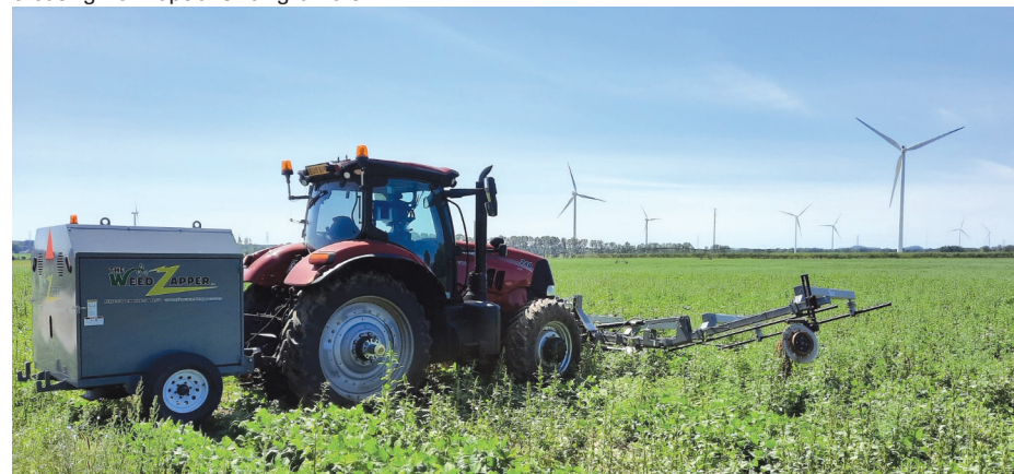
Innovation in electrical weeding equipment from companies such as The Weed Zapper is creating new options for growers.
