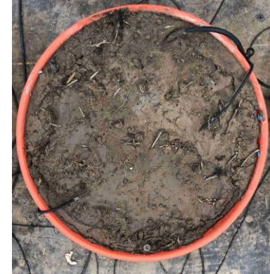
Installation of ORP sensors and irrigation
