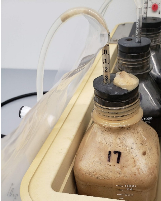
Digester 17 (soapstock) foaming excessively on May 4, 2021
