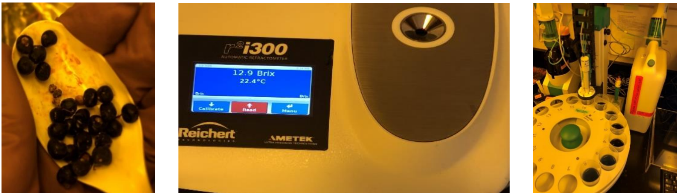
Figure 2. Stems were removed from the berries before grinding (left). Refractometer (middle) and automatic titrimeter (right).
