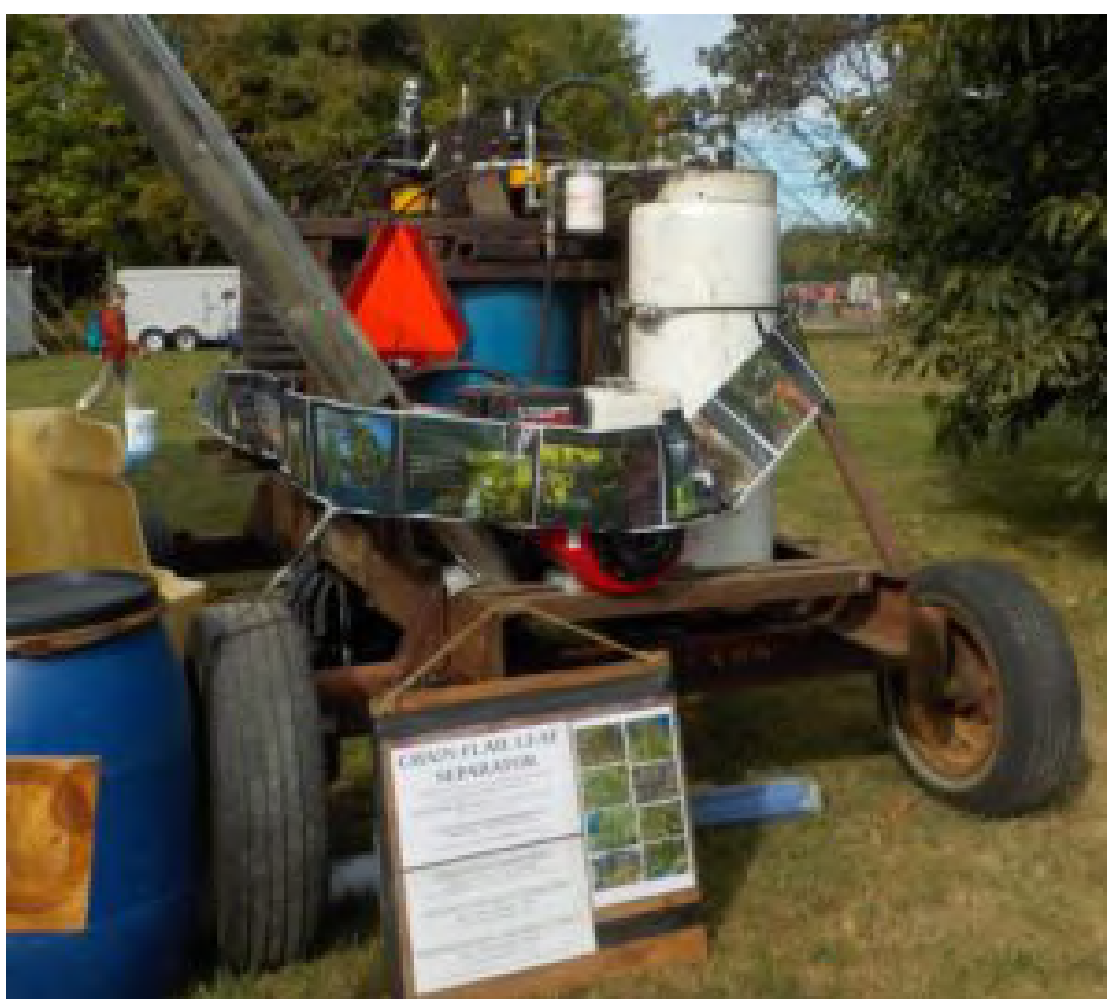
Chain-Flail Leaf-Separator, transported, repaired again (flat tire patched, re-threaded gas drain-screw, and reduced leak around the hydraulic pump, thanks to John McIntire), then set up for the 2nd year's Demo at MOFGA's 2024 Common Ground Fair
