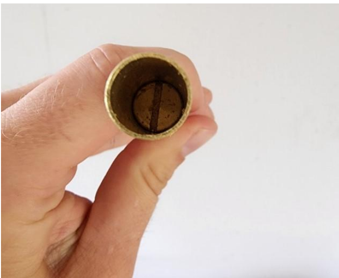
Figure 10. The inoculation tool used for sawdust spawn is a simple plunger (top left) with a chamber that is ½-inch diameter and one inch length to match the size of the inoculation hole (bottom left). The tool is inserted into spawn to fill the chamber (top right) and then the plunger is depressed to insert the sawdust spawn into the hole (bottom right). Photos: Patrick Shults, WSU Extension.
