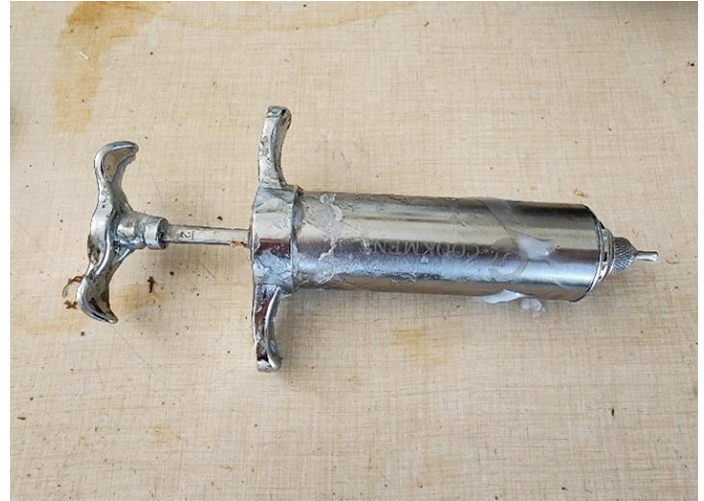
Figure 13. A hot plate with an adjustable temperature knob and a cheap pot (left photo) are easily sourced equipment for waxing. A metal meat injector with a clipped needle tip (right photo) works well for waxing and can hold enough wax to complete one or more rows at a time. Photo: Patrick Shults, WSU Extension.
