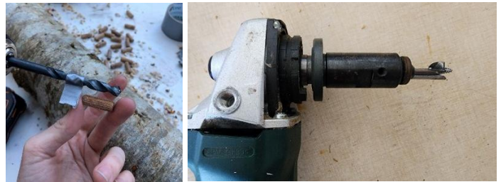
Figure 7. A 5/16th-inch drill bit on a cordless drill with a piece of tape placed as a makeshift stop for one-inch-deep holes to match the length of the plug spawn (left photo). A modified drill bit with a one-inch shoulder stop attached to an angle grinder for faster drilling (right photo). Photos: Patrick Shults, WSU Extension.
