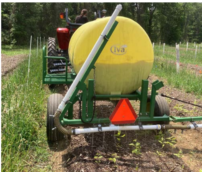
Figure 4: The Rich Earth applicator with one boom retracted, delivering urine to a bed of nursery trees at Yellowbud Farm.
