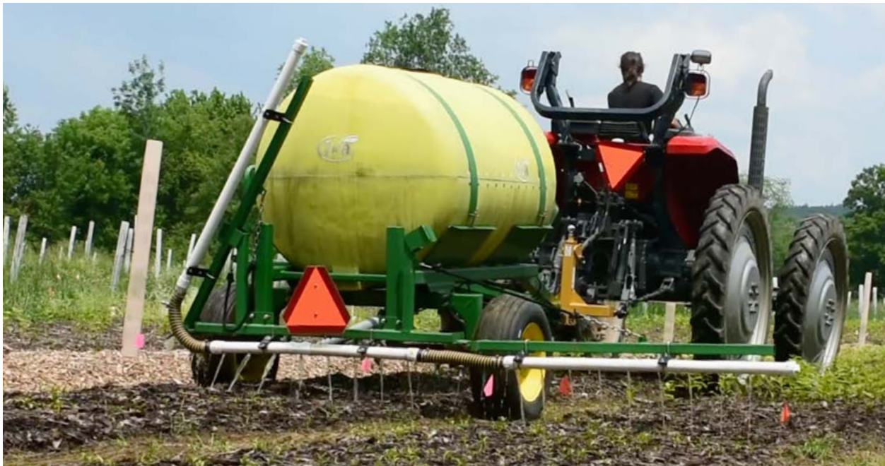
Figure 13. Rich Earth's custom field applicator applies urine fertilizer to nursery stock.
