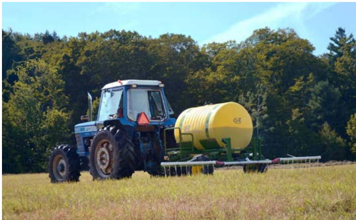
Figure 2: A tractor pulls the Rich Earth applicator, fertilizing a hay field.
