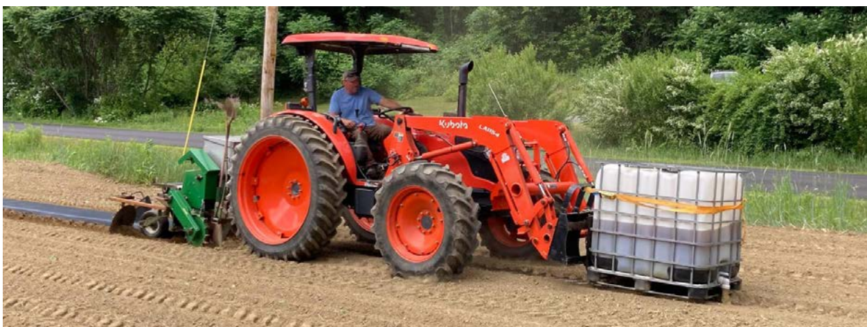
Figure 6. A tractor carries an IBC tote of urine fertilizer on forks while pulling a plastic layer from the rear
