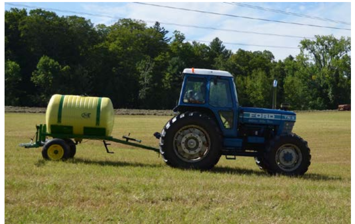
Figure 3: Side view of the Rich Earth applicator applying urine on a hay field.
