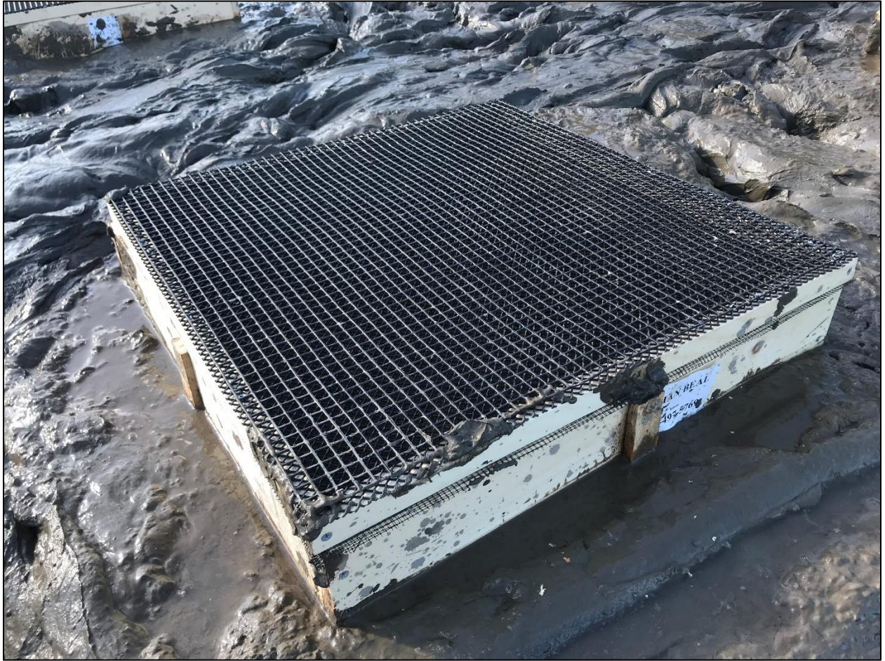
Figure 7. A 2-ft x 2-ft wooden box that contains Arctic surfclam juveniles. Wooden stakes (24-inches long) are forced into the sediment and then screwed into each side of the box. The top frame (1-inch thick) contains three different sizes of protective netting (see Fig. 6) to deter predators.
