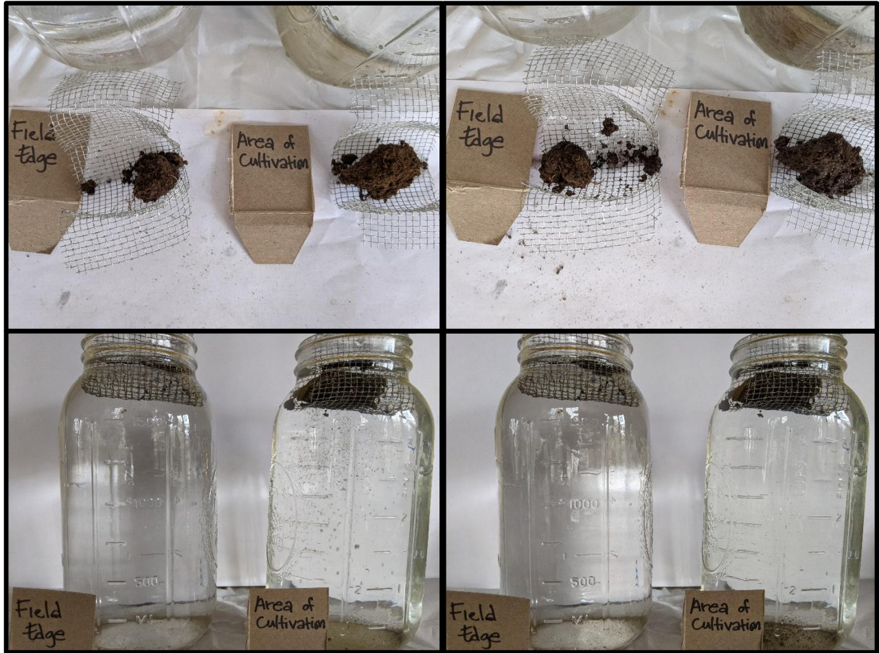
Image 1. Slake test performed on hedgerow/field edge and production field/area of cultivation at Simple Gifts Farm.
