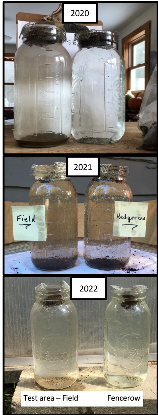
Image 3. Slake test observations for field and hedgerow over three years of sampling at Massaro Farm.
