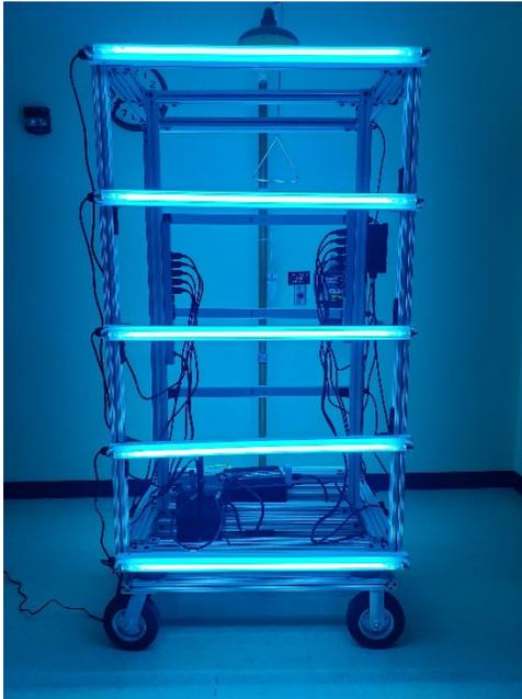
Fig. 1. UV-C cart assembled for this project with parts procured from multiple suppliers.
