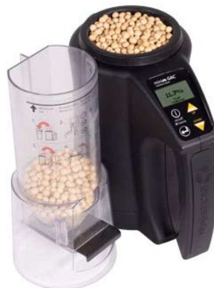
Handheld grain moisture meter
