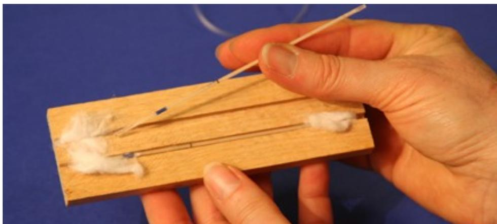
To seal the capillary tube for storage, a silicone cap or glass beads connected with pieces of silicone tubing can be used.
