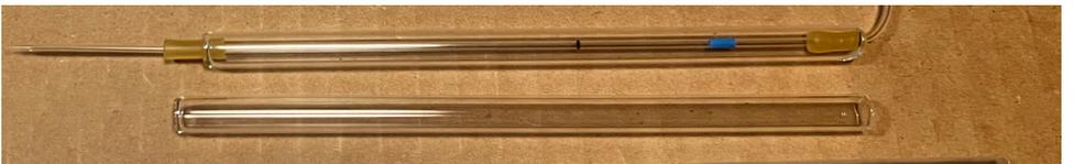
5. Pull the assembly of the capillary tube and tygon tubing through the protective glass barrel.
