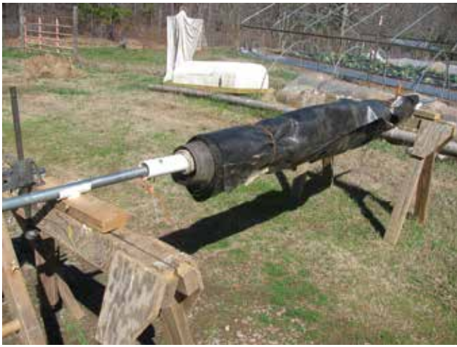
Figure 5. For labor-efficient laying and pickup of the landscape fabric, Bryan uses a landscape fabric reel consisting of a 1.3 inch diameter metal tube with a wooden handle, supported on two sawhorses. The six-foot wide landscape fabric is laid on raised beds spaced five feet center to center, overlapping in alleys and anchored with eight-inch metal staples. This method makes landscape fabric practical for his three-acre mixed vegetable operation.
