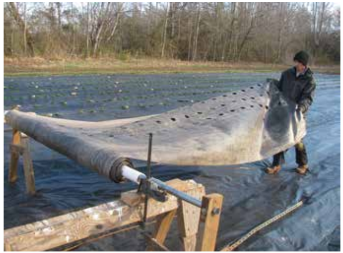
Figure 5. For labor-efficient laying and pickup of the landscape fabric, Bryan uses a landscape fabric reel consisting of a 1.3 inch diameter metal tube with a wooden handle, supported on two sawhorses. The six-foot wide landscape fabric is laid on raised beds spaced five feet center to center, overlapping in alleys and anchored with eight-inch metal staples. This method makes landscape fabric practical for his three-acre mixed vegetable operation.
