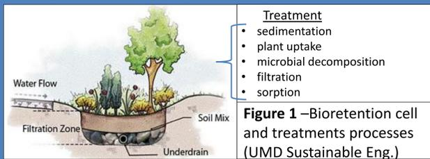
**Figure 1** – Bioretention cell and treatments processes (UMD Sustainable Eng.)
