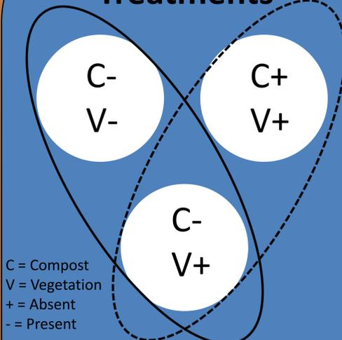
**Figure 3** – Experimental amendments of Miller Farm Bioretention Cells. Two cells were vegetated, with one cell having compost added under the planting locations. Circled cells are experimentally paired to test the effects of compost (dashed) and vegetation (solid) on bioretention pollutant removal.
