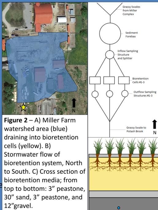
**Figure 2** – A) Miller Farm watershed area (blue) draining into bioretention cells (yellow). B) Stormwater flow of bioretention system, North to South. C) Cross section of bioretention media; from top to bottom: 3” peastone, 30” sand, 3” peastone, and 12” gravel.
