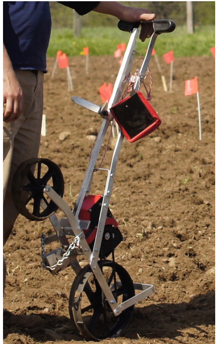
Figure 1. The push seeder is a tool used for planting row crops that comes with a row marker, seed hopper, and adjustable ground opener allowing for different planting depths. Photo by Julianne Kellogg.
