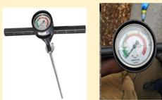
Soil compaction using a Dickey-John Tester
