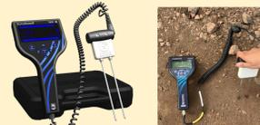
Soil moisture content using the Hydrosense II CS658 probe
