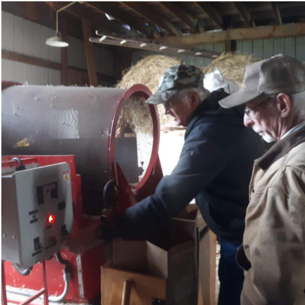
Leonard Reggie, left, and Rodney Leighow go over the startup procedure for a switchgrass chopper. The machine was built with funds from a USDA grant and chops switchgrass into a material that can be used for poultry bedding and garden mulch.
