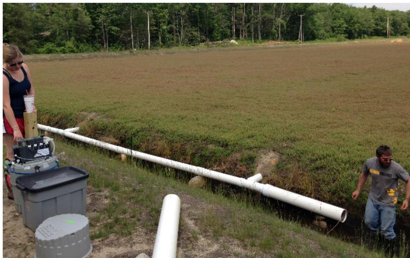
The tiles in this bed were 25 feet apart and about 2 feet deep. For two years, flow data were gathered as were samples to quantify nitrogen in the drainage leaving the tiles.
