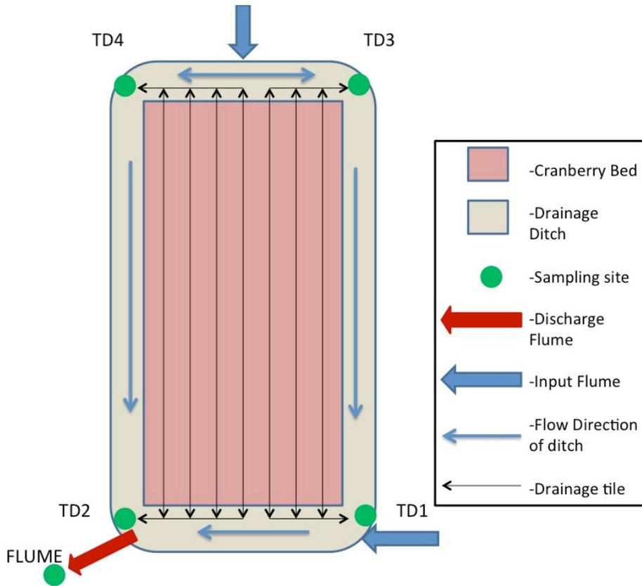
TD1-4 are groups of tiles joined by a pipe. The pipe is used to connect groups of drains that can then be sampled using automated equipment. See the picture below.
