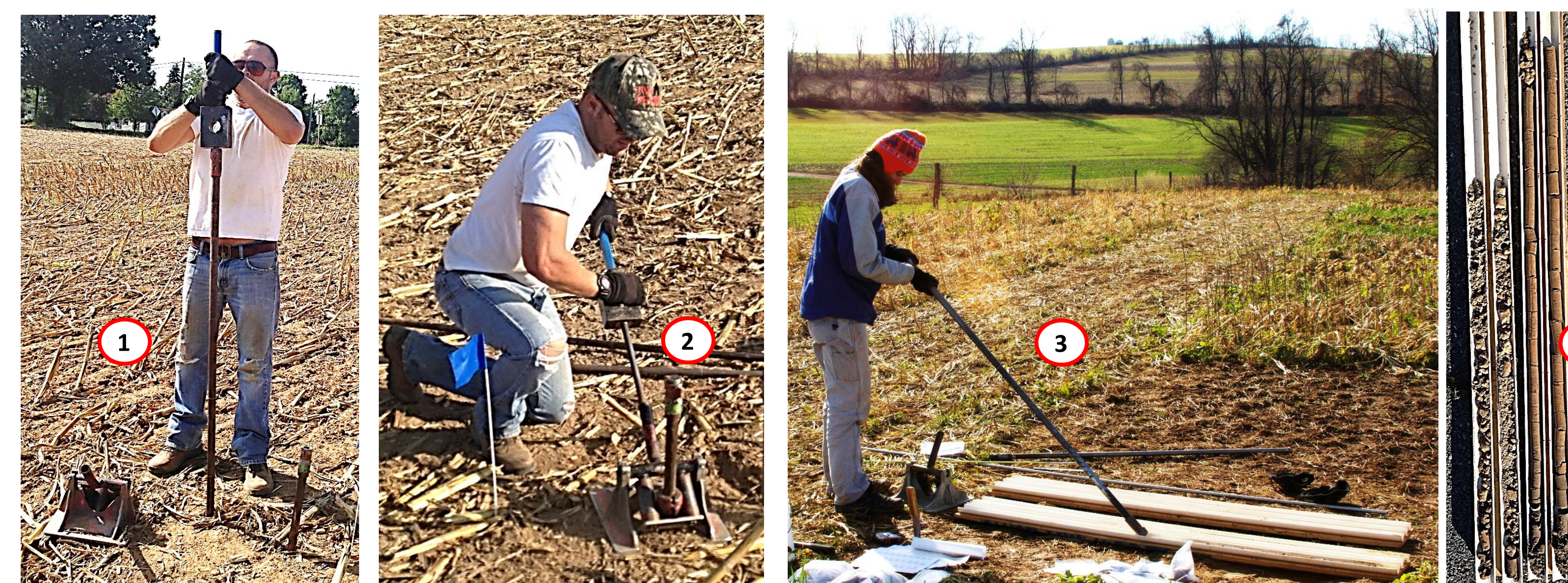
Figure 4. Procedures for taking deep soil cores using Veihmeyer probes (photo 3 taken during early spring sampling, data not shown)
