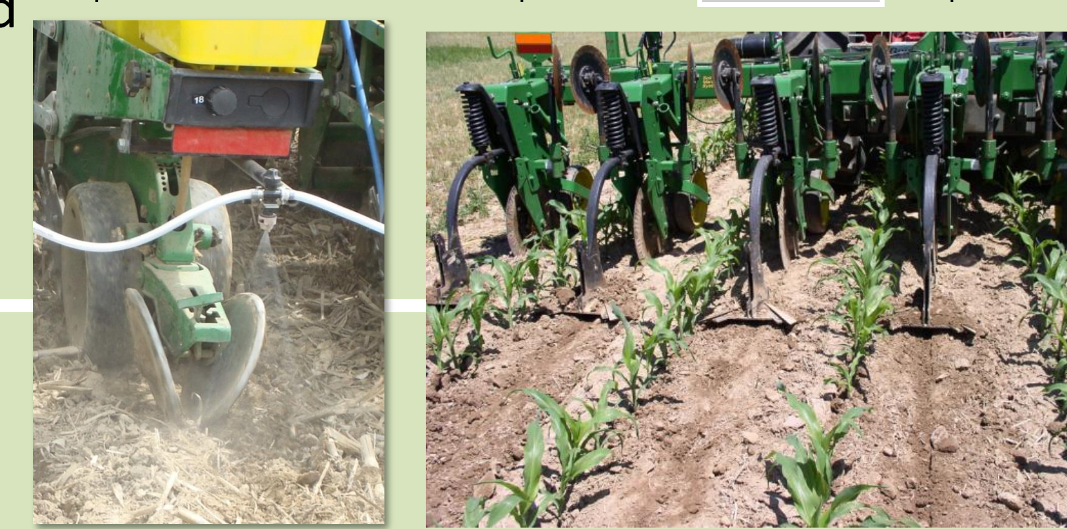
Banding herbicide over the crop row (left), using high residue cultivation post (right).
