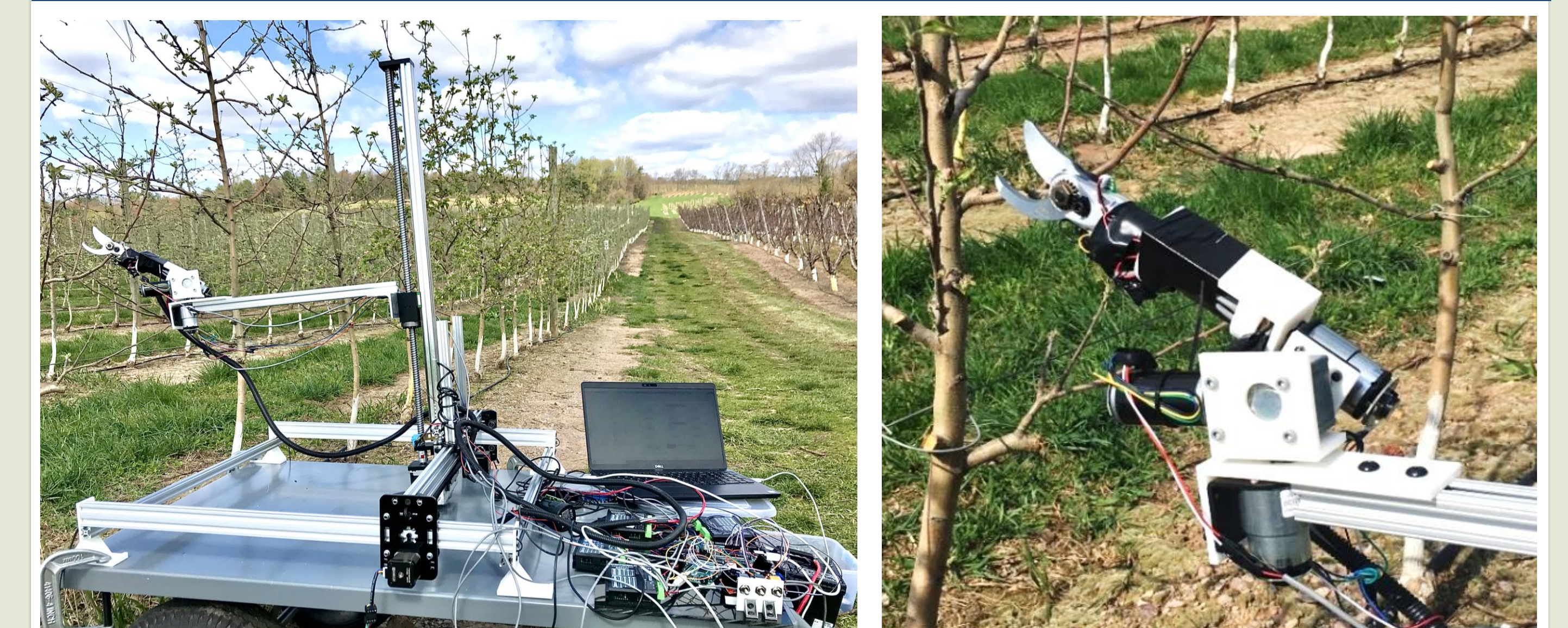
Fig.7.(a) Experimental setup in the field; (b) Robot end-effector
