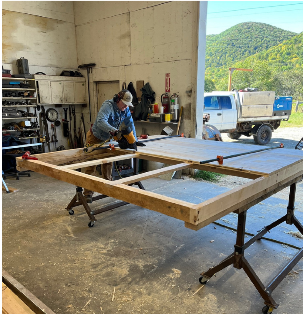
Exterior Wall Claddings being batch manufactured at The Locust Works. The role of the cladding is primarily weatherization and supplemental insulation. As previously mentioned, wall shear is provided by the heavy corner brackets comprising the Core Frame.
