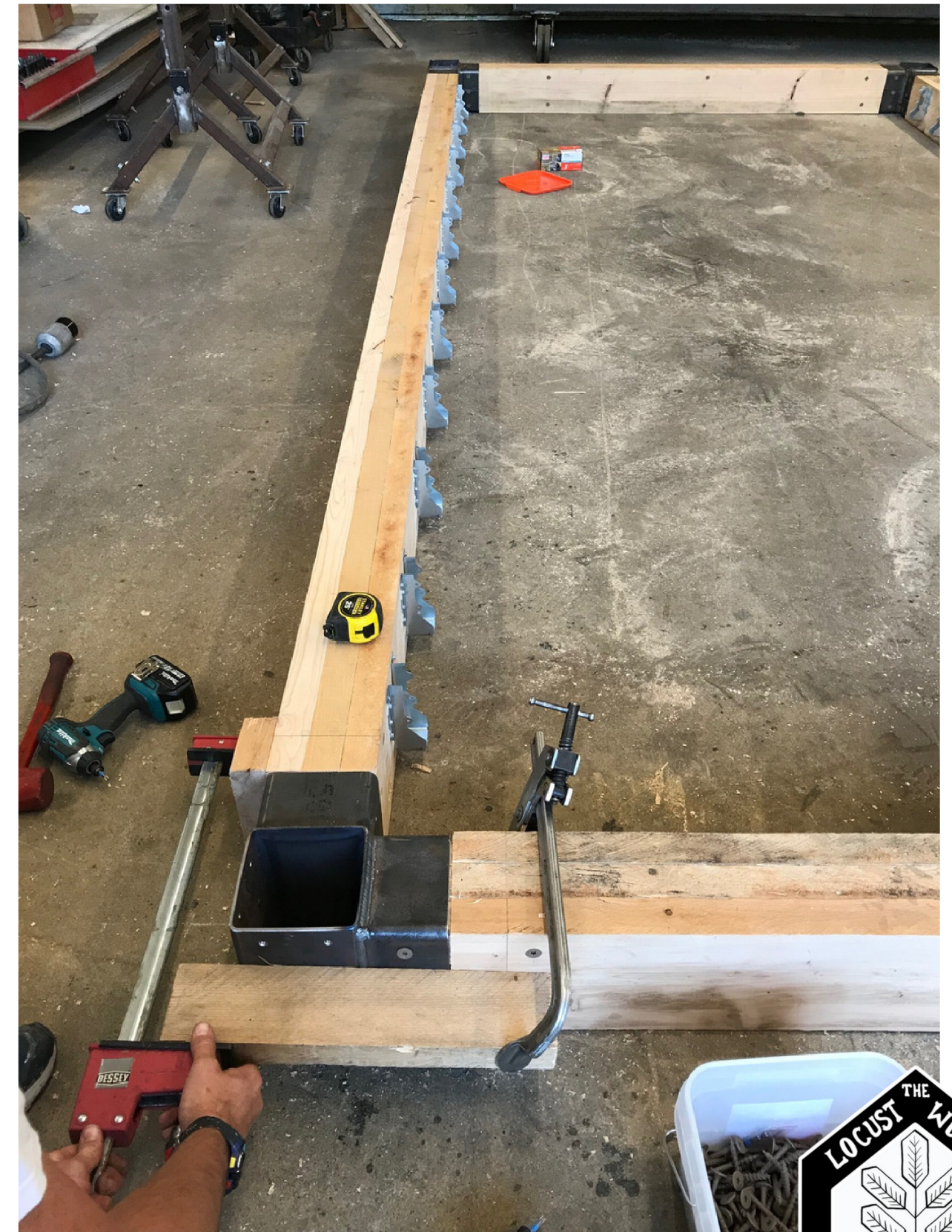
The Corner Brackets are weldments that can be fixtured and welded to close tolerances. If the timbers are carefully cut to length and pulled in tight to the brackets as shown, the ModAPS units come together very square.
