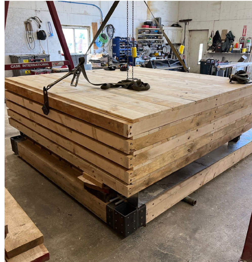
Exterior Wall Claddings being batch manufactured at The Locust Works. The role of the cladding is primarily weatherization and supplemental insulation. As previously mentioned, wall shear is provided by the heavy corner brackets comprising the Core Frame.
