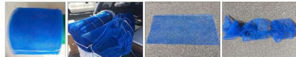
**Netron (above)** is a stiff but flexible blue plastic mesh that comes in 300 foot rolls. Other materials such as 1/4" black agricultural netting also work for spat collection, and more cheaply. Each spat bag will need three pieces of Netron cut to 17" x 30", or 20-40 square feet of material. These materials can be re-used for a number of years.
