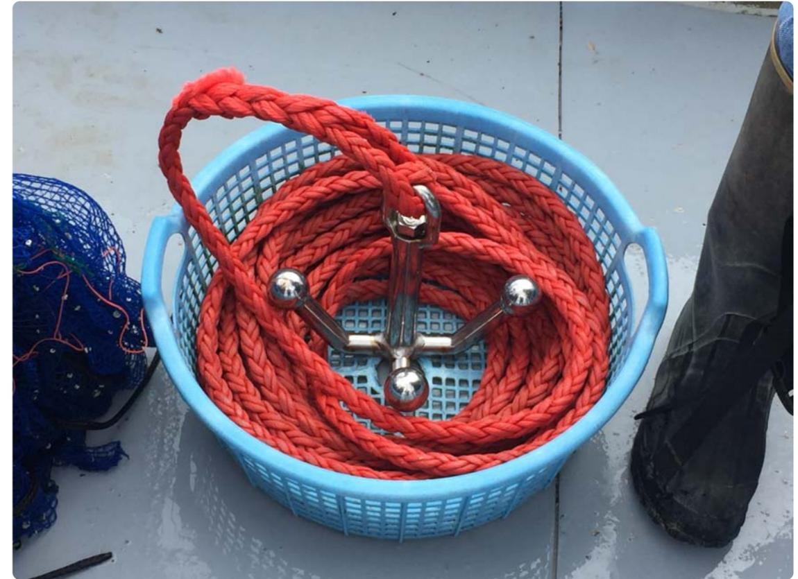
*Grappling Hook used to secure long line to vessel*
