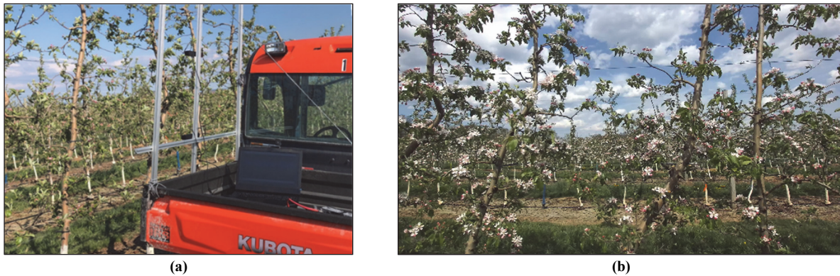
Figure 3. (a) Image acquisition system mounted on a Kubota utility vehicle; (b) example of acquired images in a trellis-trained tall spindle apple orchard.
