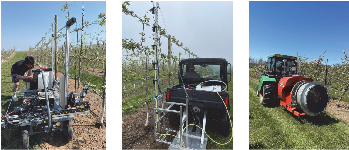
Figure 7. Spraying systems used in the test. Left: Cartesian target sprayer (CTS); middle: boom-type sprayer (BTS); right: air-blast sprayer (ABS).
