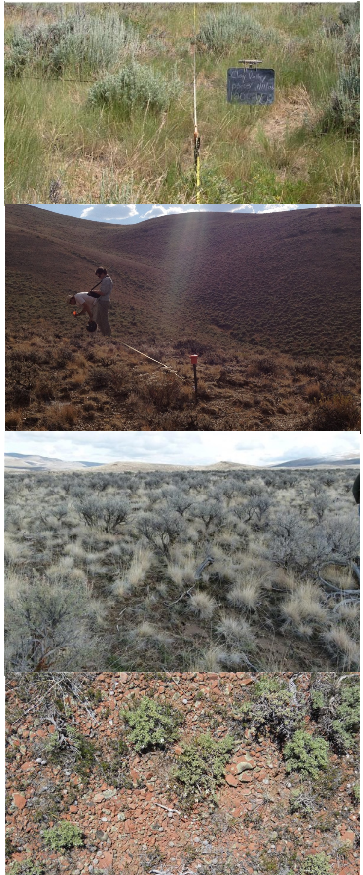
Figure 27. Canopy cover is often measured with a stretched measuring tape using either line intercept or line point intercept, which is often used for foliar, basal or ground cover.
