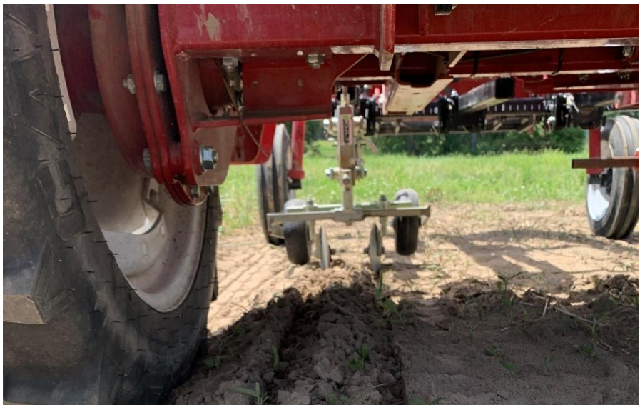
Figure 2.1. Image of cultivation tools used in experiment, including a) finger weeders (Tilmor) and b) hilling disks (Kult Kress 'Duo' cutaway disks set to hill).
