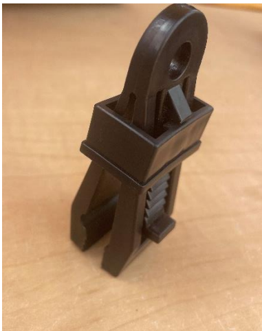
Figure 3.2. Tarp clip (Outus brand “crocodile mouth” tarp clip) used to connect plants to force gauge for anchorage force measurements.
