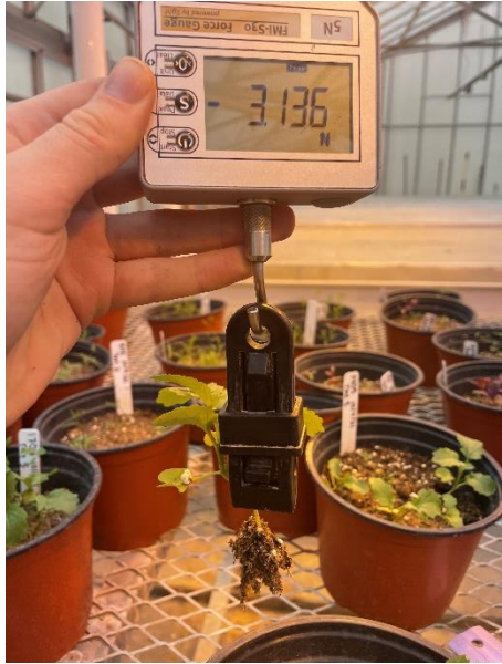
Figure 3.3. Anchorage force gauge (Alluris FMI-S30) shown uprooting mustard seedling.
