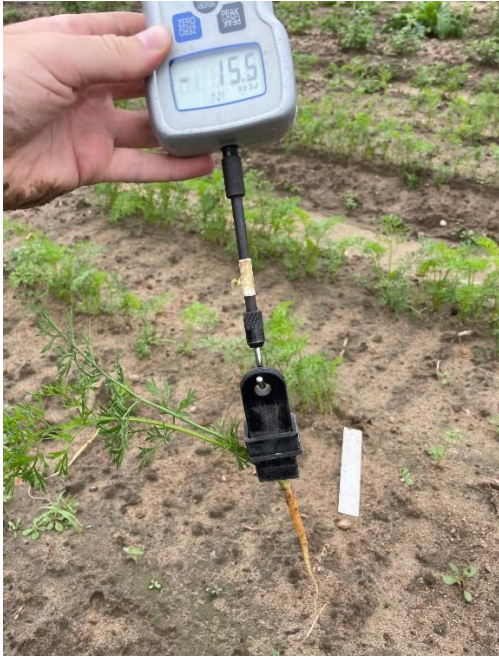
Figure 2.2. Anchorage force gauge used to uproot plants.
