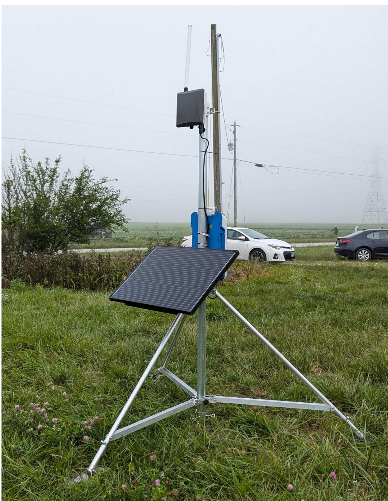
Gateways in fields or on facilities provide LoRaWAN connectivity and pick up LoRaWAN device data
