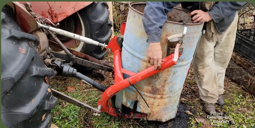
Image 1: PTO driven walnut huller made out of an old lime spreader and steel drum.
