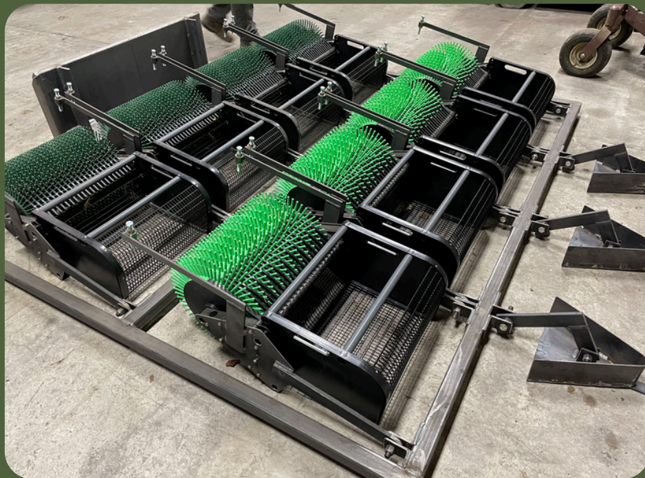
Image: Tractor mounted ground-nut collector based off the bag-a-nut. Image Credit: Bob Stehli, Wintergreen Tree farm
