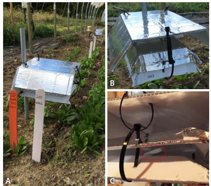
Figure 14. A. Homemade radiation shield in use in a high tunnel. B. Close-up of radiation shield shown in A. C. Close-up of radiation shield showing location of temperature sensor between bottom and second layer of shield.
