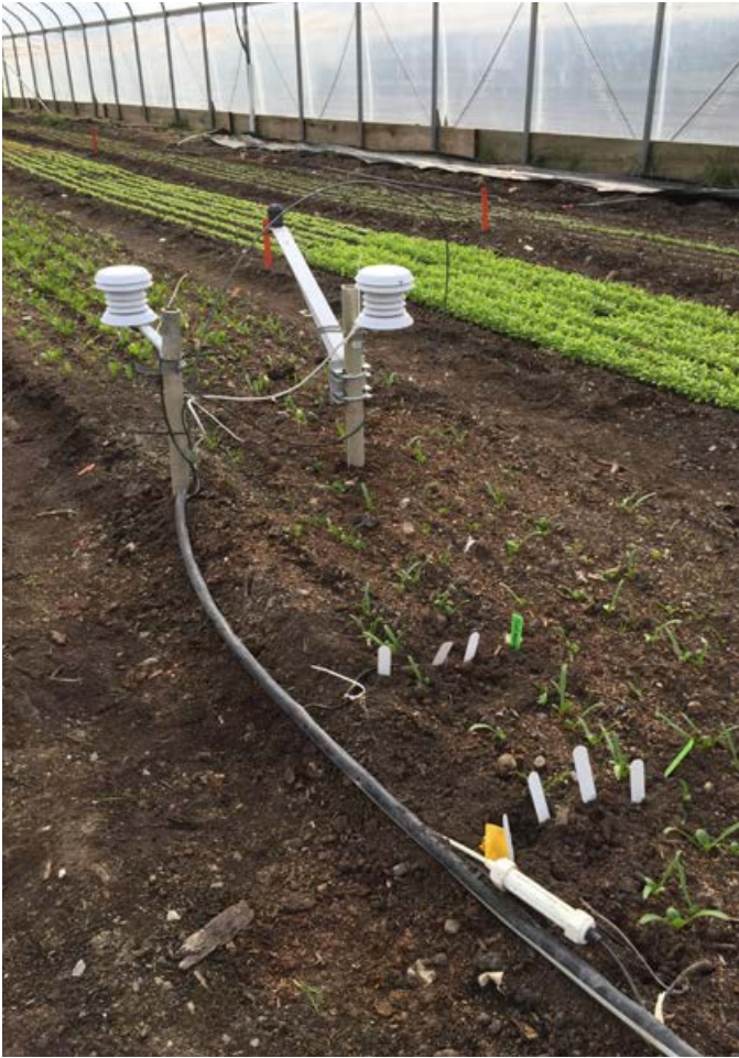
Figure 13. Temperature sensors inside the white radiation shields are installed so that when row cover is placed over the hoop one sensor will be underneath the cover, and one above the cover. Also visible is a light (PAR) sensor that will be underneath the row cover. The white pot labels in the foreground mark cables leading to buried temperature and soil moisture sensors. (Photo by E. Maynard)
