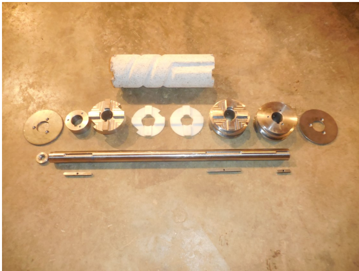
Here are the components of the main shaft assembly.
