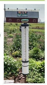
*Figure 2. Example of an atmometer.*
