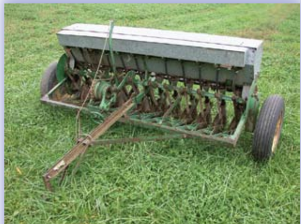
A small seed drill works well for planting cover crops
