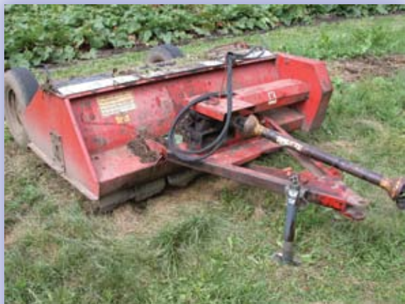
A flail chopper works well for clipping cover crops
