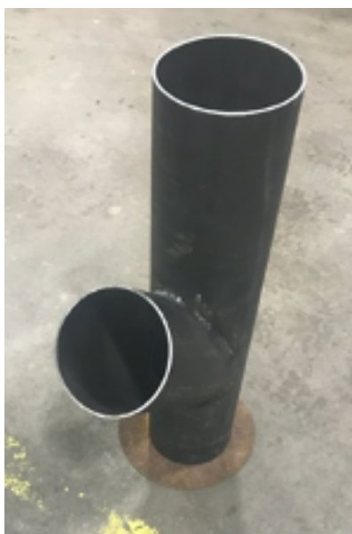
Figure 1 – The chimney and wood feed
