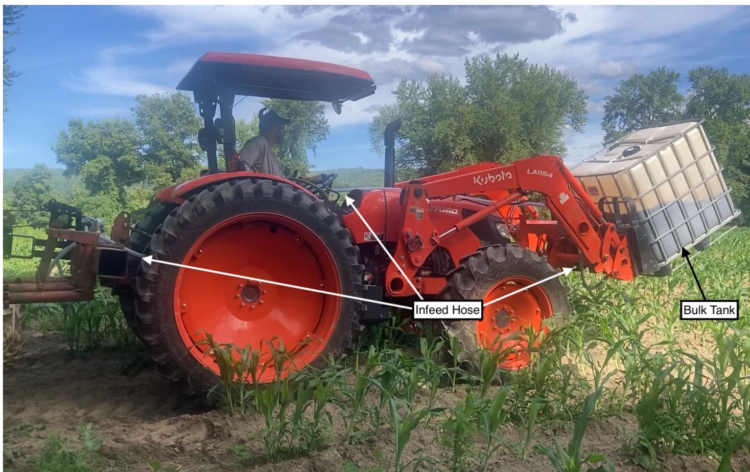
Photo 1: IBC on front forks with infeed hose bringing urine from front to back of tractor to the roller pump.
