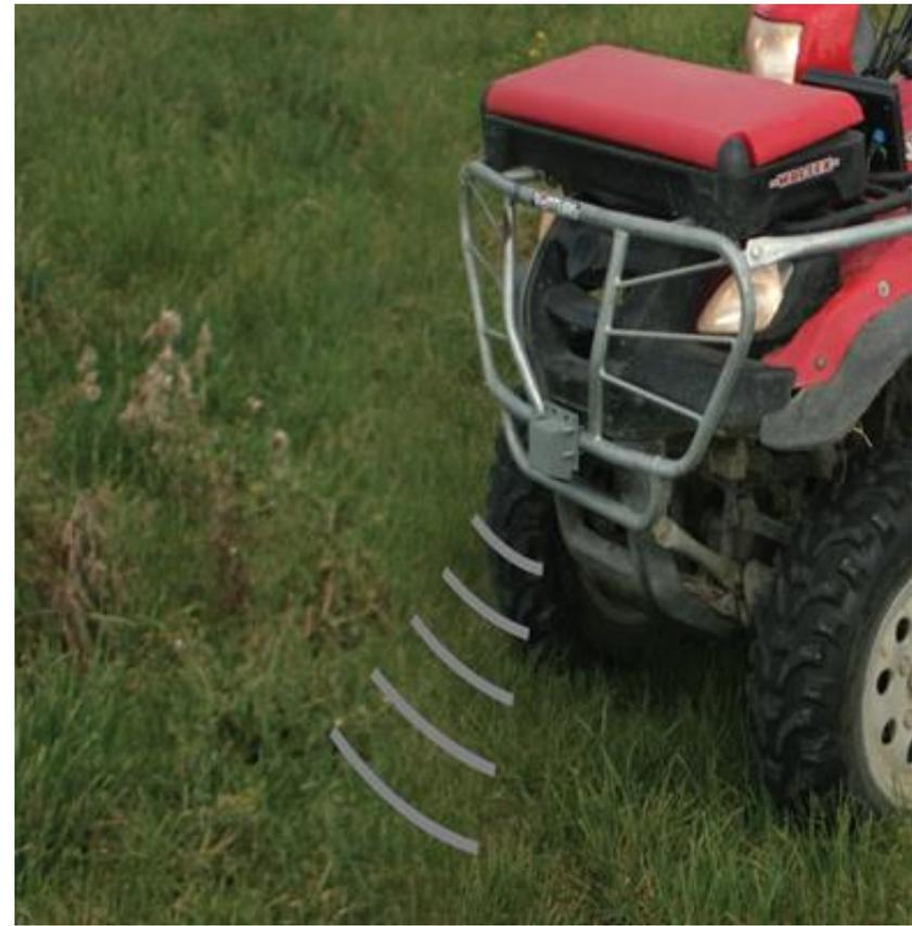
Calibrating Red River Crabgrass by harvesting known area and calculating kilograms of dry matter forage per square meter. Height of the forage is measured by use of the sensor technology (20 readings per second).
