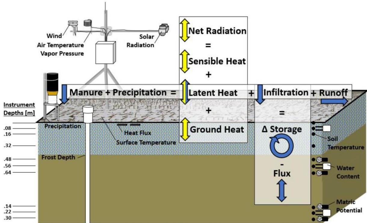
**Figure 3.** Schematic of the measured soil, hydrological, and atmospheric parameters, which allow for the quantification of infiltration capacity, runoff, and energy available for melt. Not pictured: passive, divider runoff collection equipment with load cells and snow sticks for snow depth measurements.
