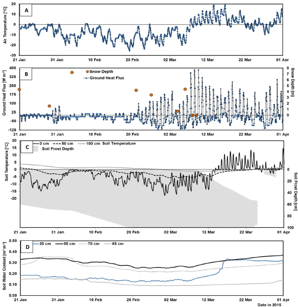
**Figure 6.** A sample of the key parameters for the water-energy balance, measured in the absence of manure during late winter 2014-2015 (pilot season). A) Air temperature, B) Ground heat fluxes and snow depth, C) Soil frost depth plotted with select depths of soil temperature, and volumetric water content. Data were collected hourly, with the exception of soil frost and snow depths, which were manually collected daily to weekly.
