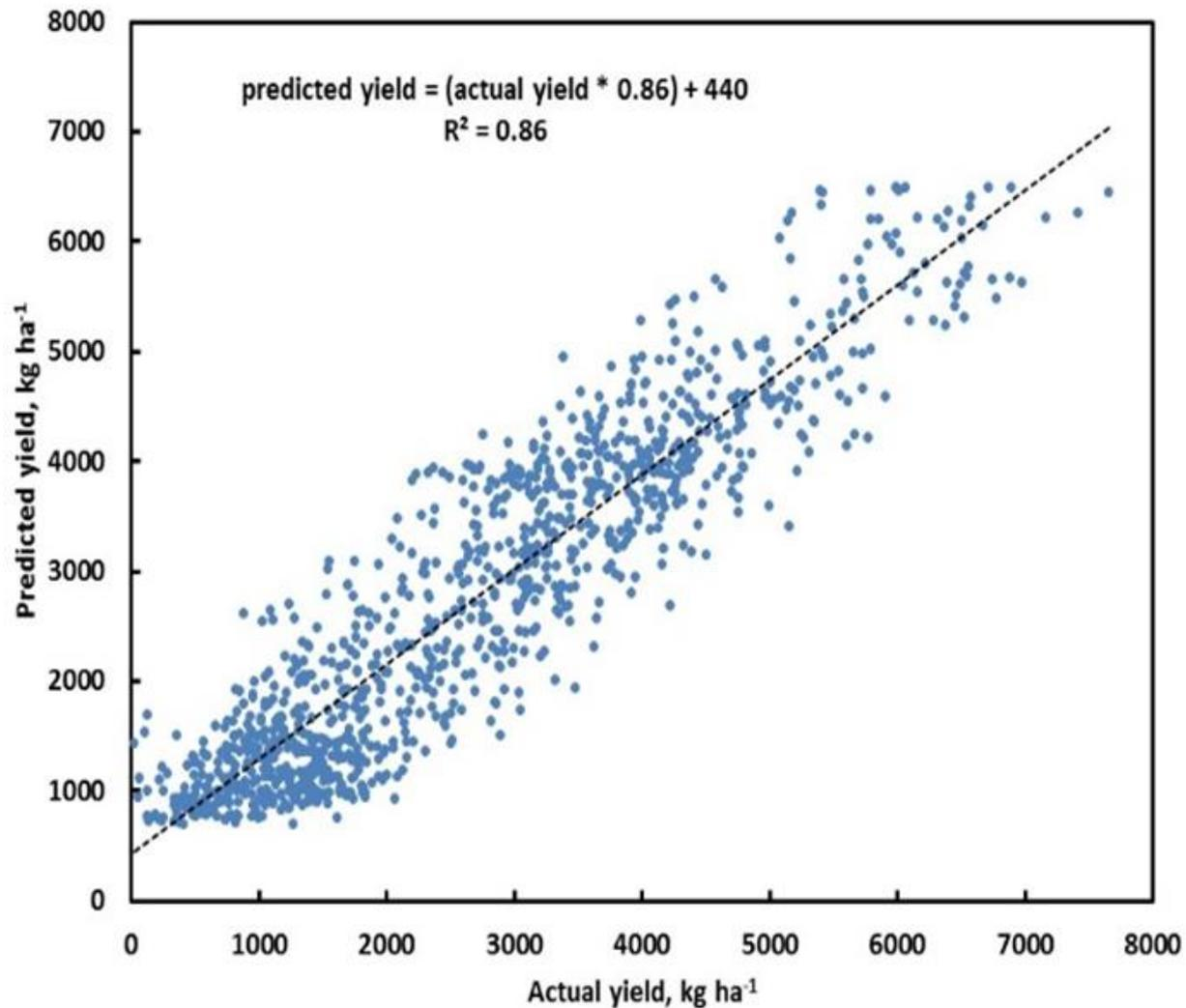
Figure 3. Linear relationship between actual forage yield and that predicted by the ultrasonic sensor modeled with other environmental parameters. Data collected over 19 site-years provide the basis for introducing this technology on farms.
