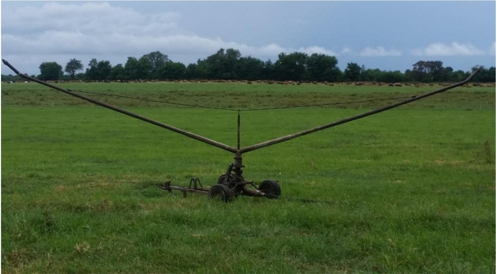
Figure 9: Low-pressure traveling gun (Spider). Irrigator is pulled across the paddock via a cable and ratchet powered by water pressure turning the arms. The water line is pulled behind the irrigator. This can limit the type of forage species irrigated due to the water line
