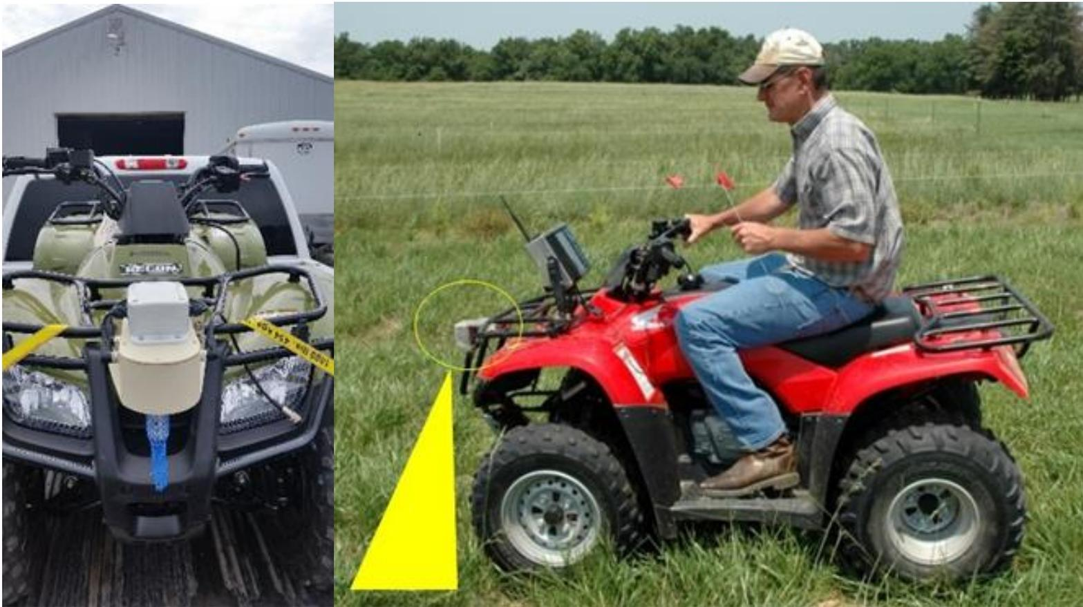
Figure 1: Front-mounted Senix sensor system implemented on ATV for measuring pasture height. Sound waves from the sensor reflect off the forage. The time difference between the tare value (zero) and forage indicate forage height in mm.
