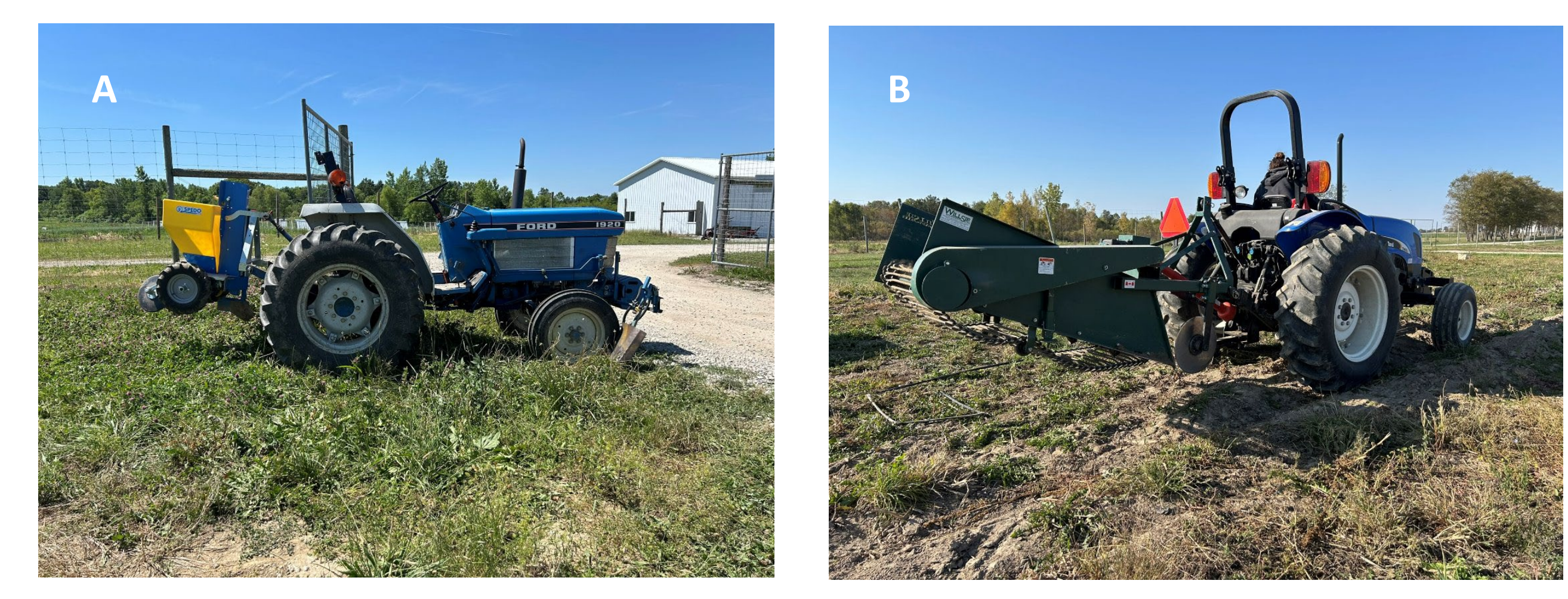
Figure 2b. Tractor traction field activities from the side-by-side, randomized and replicated tractor-animal traction comparison at the Meigs Horticulture Facility 2024. A). Tractor and potato planter used for planting in the tractor traction treatment; B). Tractor and potato digger for harvesting potatoes in the tractor traction treatment.
