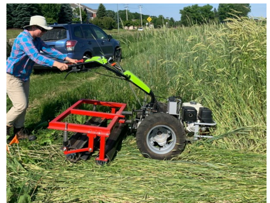
Figure 1: Rue Genger tests out the crimper on a stand of rye at West Madison Agricultural Research Station
