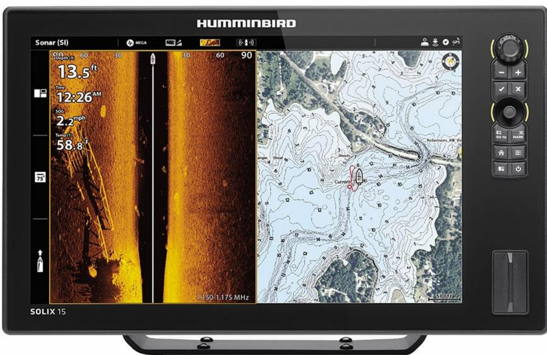
Example of a sidescan image (left side) and navigational aid (right side) in a split plot display on a Humminbird Solix 15 Fish Finder
