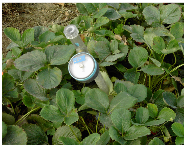
Photo 6-4. A tensiometer is an easy-to-use low tech tool for monitoring soil moisture levels (D. Handley).
