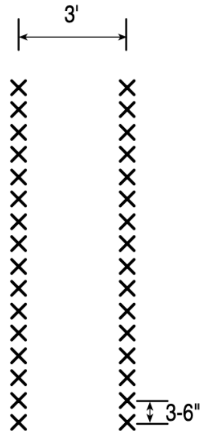
Figure 4-3. Spacing diagram for the ribbon row system.
