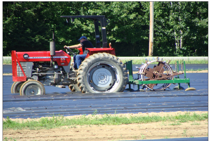
Photo 4-35. Dibbler wheel used to mark the correct plant spacing and create holes for planting (D. Handley).
